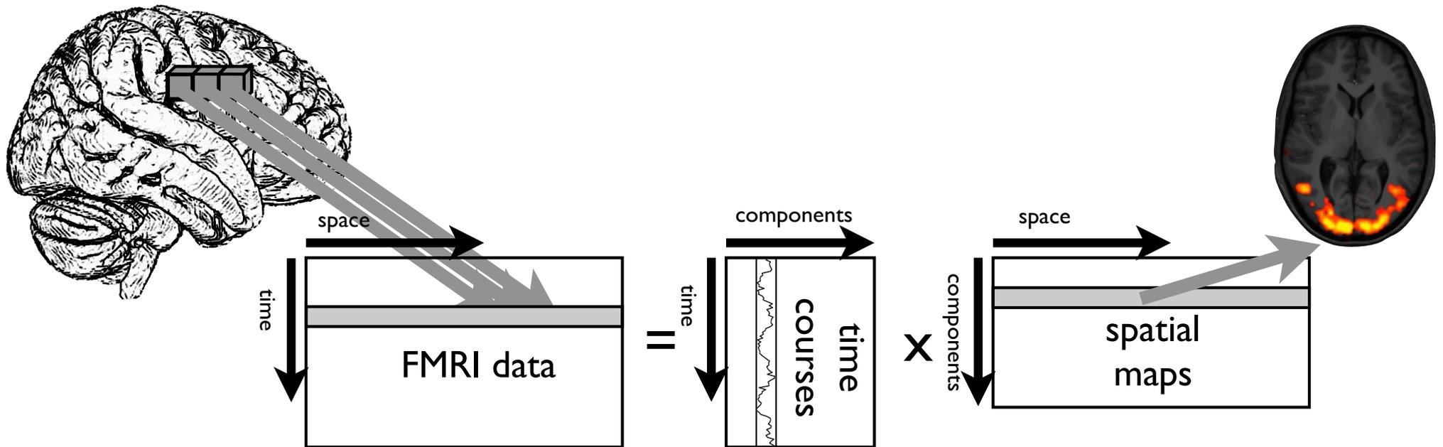
Data is represented as a 2D matrix and decomposed into components
