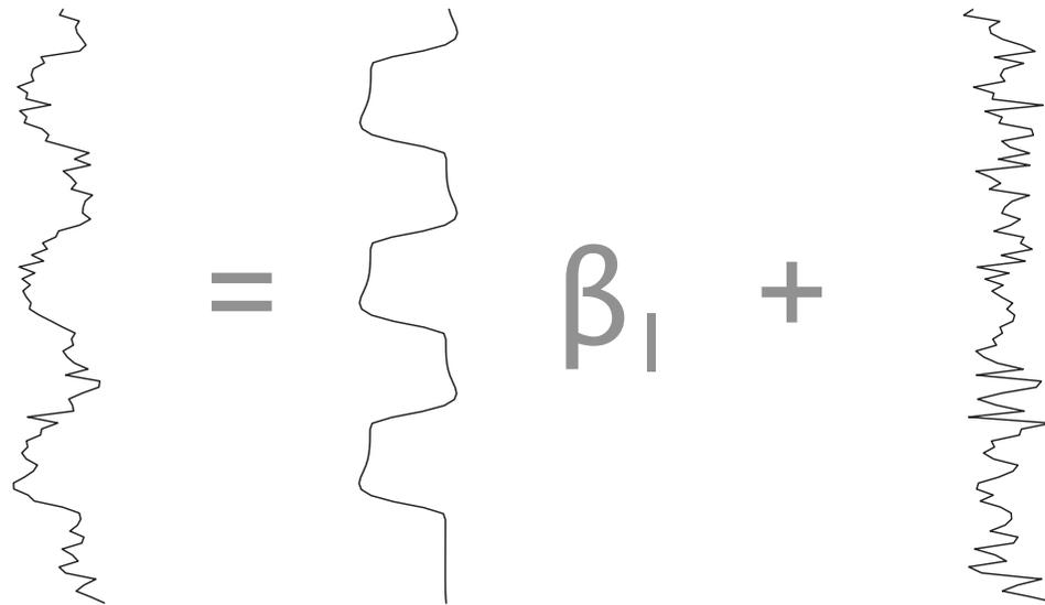
The diagram illustrates the General Linear Model (GLM) equation. It shows three vertical time-series plots. The first plot on the left is a noisy signal. This is followed by an equals sign, then a second plot showing a smooth signal multiplied by the Greek letter beta with a subscript 1 ( $\beta_1$ ). This is followed by a plus sign and a third plot showing a noisy signal. This visualizes the equation: measured time-series = signal  $\beta_1$  + noise.
